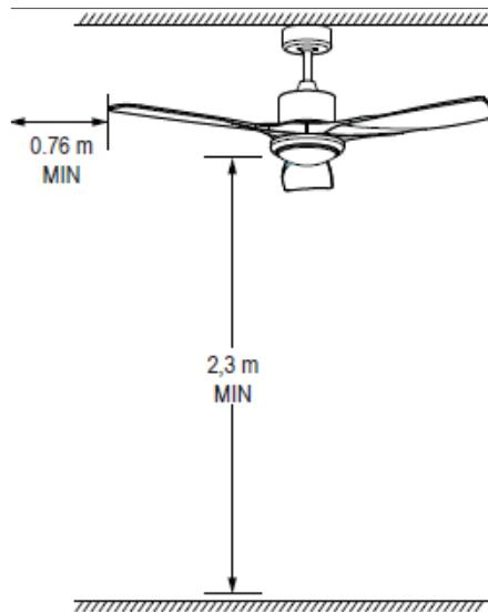
CAUTION: Before installing the fan, be sure to turn off the power. Do not switch on the power supply until the fan is fully installed and ready for use.
